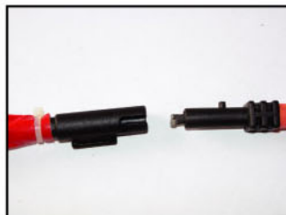
Manual Fuse disconnected from E-Link Connector
