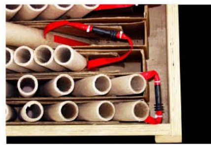
Individual Modules linked together using the Fire Transfer Connectors
