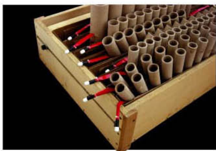
Modules being loaded. Each row is equipped with an E-Link Electric Match Connector
